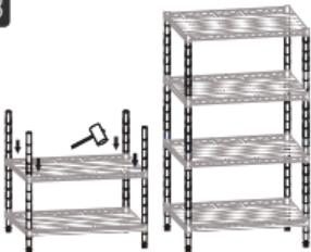
Use the four middle poles to spiral tighten clockwise with the bottom poles. Repeat the previous steps to install the second and subsequent layers.
