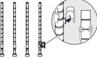
Take out the four bottom pole with feet. Secure the plastic clips at the same height on each pole. It will utter a sound while installing well the clip. (Set the height according to your needs, making sure the "TOP" side of the clip faces up.)
