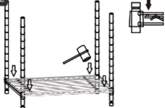
Slide the wire mesh onto the four poles, stand it up, and gently tap the connections to secure them.
