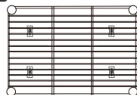
Thread plastic ties through the metal clips and secure the clips to the wire mesh.
