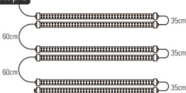
Connect the lights as shown, ensuring the correct positioning of the 35 cm and 60 cm connection cables. Install the waterproof cap on the last light bar.
